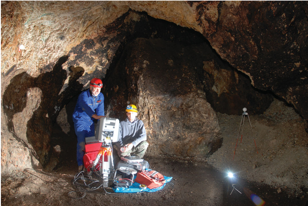
Figure 2. Recording the prehistoric Fahlore mine at Mauk E with laser-scanning techniques.
