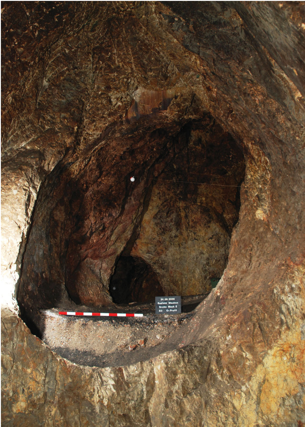
Figure 3. A typical round hollow resulting from extraction of ore by fire-setting (at Mauk E, eighth century BC).
