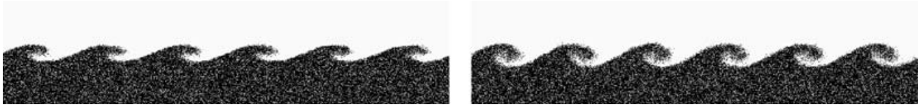
Figure 15. A zoom in of the SPH particles at the boundaries between the shearing layers for the isodensity SPH run with standard viscosity (left) and low viscosity (right) at \tau_{KH} . The black and white regions are particles that belonged to the initially separated shearing layers. We clearly see growth of the KHI in the standard implementation of SPH, and even stronger for the low viscosity version. The simulation was performed with GASOLINE using 10^6 particles in the same way as SPH3 described in Section 6.2.
