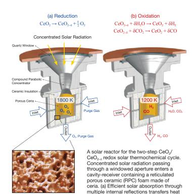
endothermic reduction, releasing oxygen. (b) Reacting gases H<sub>2</sub>O and/or CO<sub>2</sub> flow radially across the porous ceria to drive the exothermic oxidation, while product gases H2 and/or CO exit the cavity through an axial outlet port. Inset: Ceria RPC. Courtesy of ETH Zürich.
