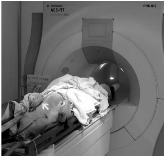
Figure 1 The animal was placed feet first, lying supine, into the scanner. It was possible to interrogate and program the pacemaker using a modified programmer head (white arrow) in the position shown above. For stimulation threshold measurements, additional ECG cables were connected to the four legs. During MRI measurements these ECG cables and the programmer head were removed due to safety reasons. During the whole time in the MRI room, the pig was monitored using the ECG from the MRI unit.
