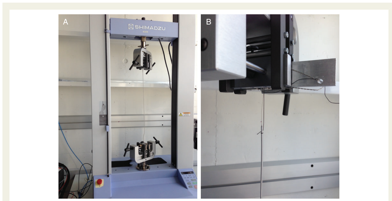
Figure 1 (A) Experimental setup of traction force testing with the use of the Shimadzu AGS-X 5 kN load cell tensile testing machine (Shimadzu). (B) The proximal part of the locking stylet was fixed rigidly to an especially constructed rectangular fixation block ( 120 \times 24 \times 4 mm).
