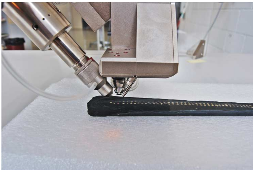
Fig 9. Experimental set-up of the micro-XRF analysis using the ARTAX 800 system. Photograph: Katja Hunger
