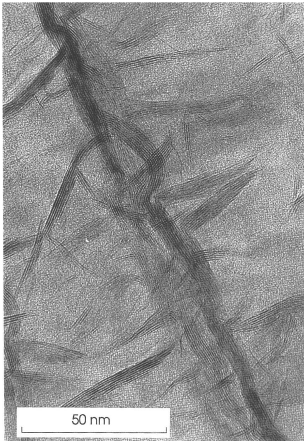
FIG. 8. Cross-sectional TEM micrograph of \text{MoS}_2 crystals in the bulk of the film, showing the dendritic-like structure induced by the branching processes.
