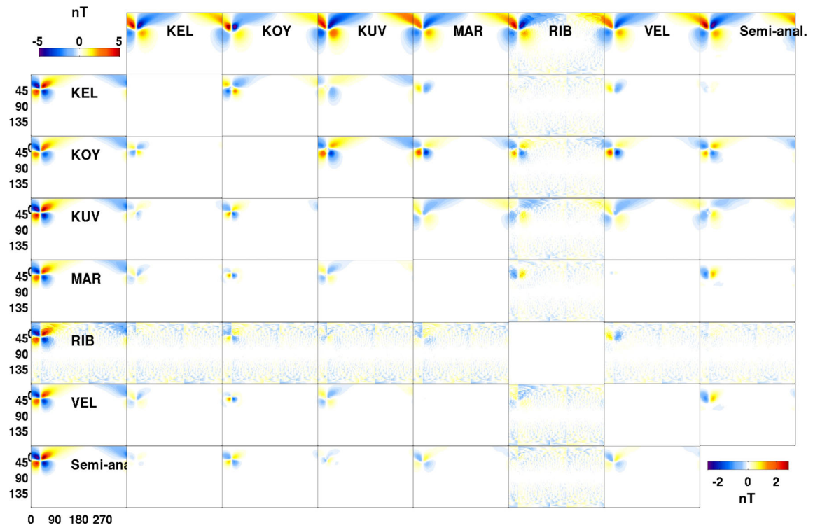
Figure 10. Real and imaginary parts of the \phi -component of the magnetic field for benchmark case 3 at a single period (1 d). The first (vertical) column corresponds to the real part of the magnetic fields. The colourbar at the top corresponds to the real part. The first (horizontal) row is the imaginary part. The colourbar at the bottom corresponds to the imaginary part. The lower triangle are the differences between the real parts from different codes. The upper triangle are the differences between the imaginary parts from different codes. The diagonal is empty. The colour scales used for the differences have the same ranges as the corresponding real/imag parts but they are shifted to be centred around zero.
