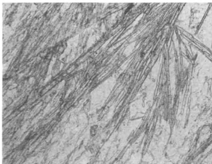
FIG. 8. Microphotograph of margarite in sample KAW 643 (Table 10). Plane polarized light. Length of picture corresponds to 0.7 mm.
