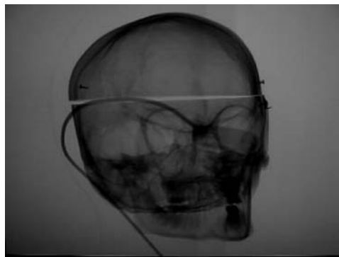
Figure 1. Reconstructed 3D image of the empty skull phantom with the XperCT system showing the position of the Radcal ion chamber close to the petrous bone.
