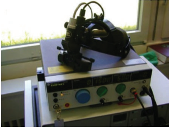
Figure 3 Indirect diode laser ophthalmoscope (DioVet®; IRIS Medical Employment, Den Haag, The Netherlands).
