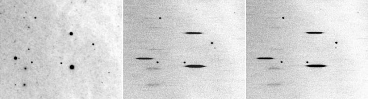
Figure 1. A sample of PN.S data. The left-hand panel shows a conventional [O III] image of a small section of M31 (M02), while the two right-hand panels show the same field as seen through the two arms of the PN.S. Note how continuum objects are dispersed into ‘star trails’, while [O III] emission-line objects remain as shifted point sources.
