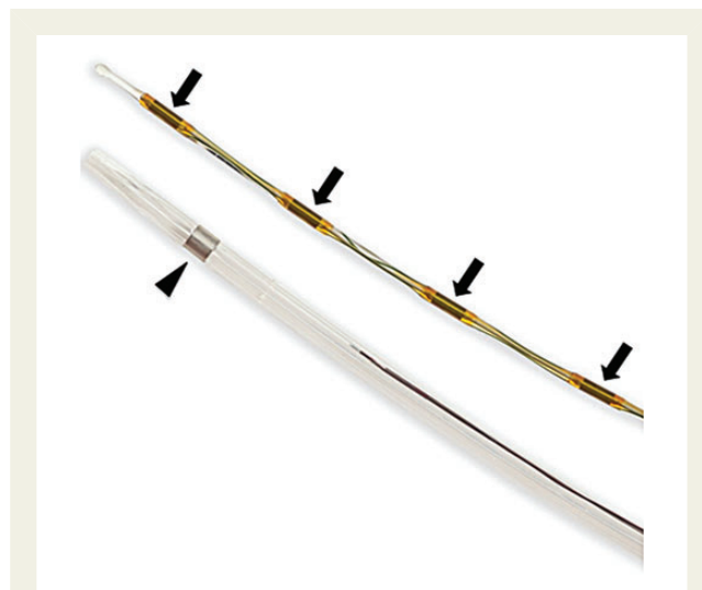
Figure 1 Tip of the ultrasound-assisted thrombolysis catheter, EkoSonic ® Endovascular System (EKOS Corporation; Bothell, WA, USA). The catheter is composed of a 5.2-Fr multi-sidehole drug infusion catheter (treatment zone marker delineated with an arrow head) and a microsonic core wire containing the ultrasound elements (marked with small arrows). During ultrasound-assisted thrombolysis, the multi-element ultrasound core wire is placed inside the infusion catheter.
