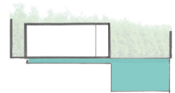
Step 6: The water reservoir and swimmingpool cool down the air, which is used for the ventilation of the house
