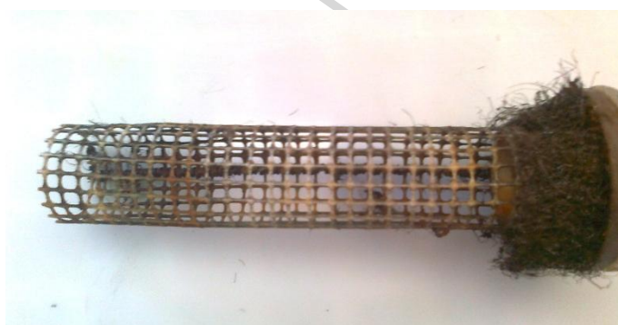
Figure 6. Picture of the exhausted anode at the end of the long-term experiment.
