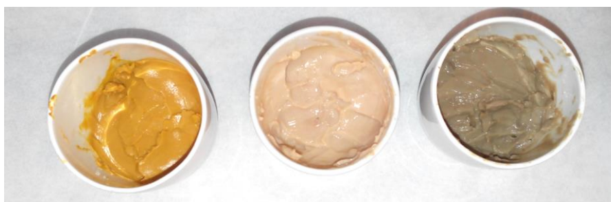
Figure 12. Paste format of hybrid composite-pigments before heat treatment. From left to right: hybrid pigments from Fe, Co and Mn salts.
