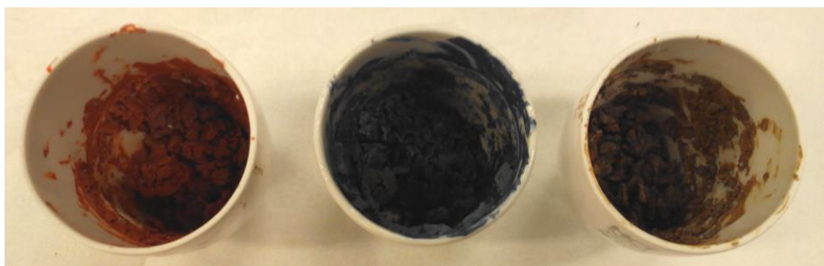
Figure 13. Powder-format of hybrid composite-pigments after heat treatment (800 °C, 3h). From left to right: pigments from Fe, Co and Mn salts.
