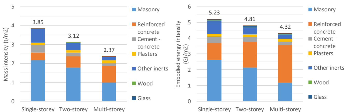
Figure 3 Mass intensity and EE intensity per floor surface unit of different archetypes (reference case).
