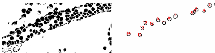
Figure 9-6. (a-d) Binary ROI - B&W images and corresponding particle analysis of Cu-PCE1, 2, 4 and 7, respectively.
