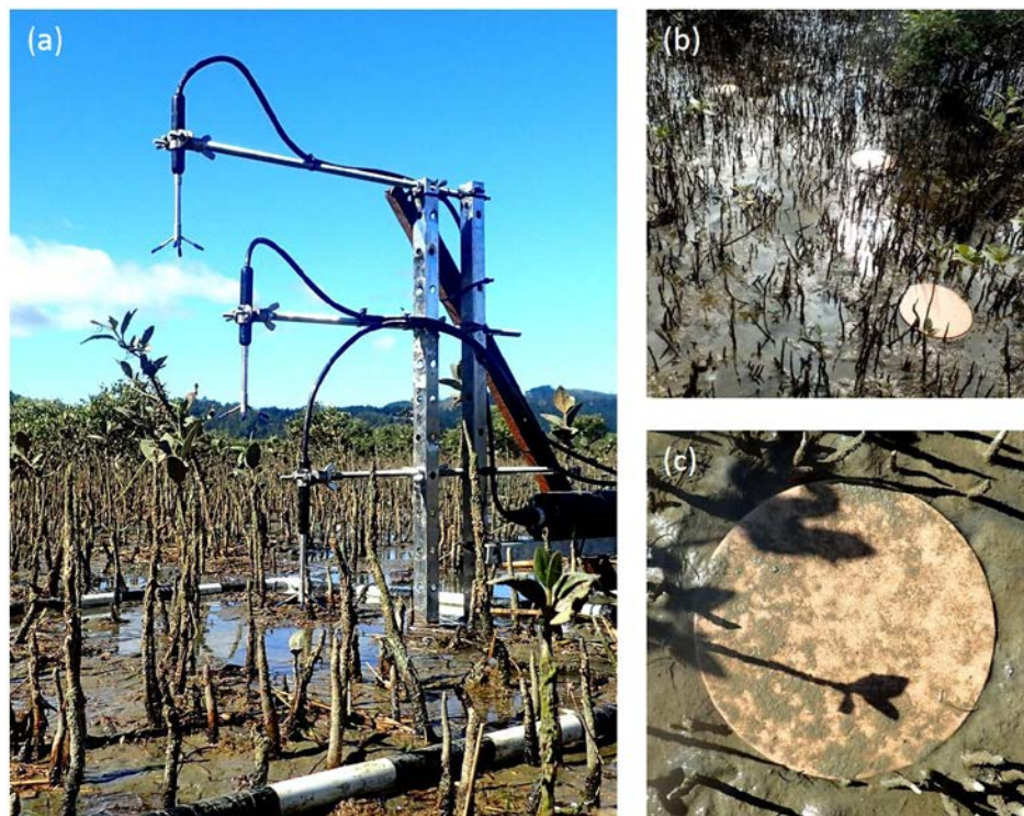
Figure 3. Field instrumentation in the mangrove fringe (around station 5 in Figure 2): (a) three vertically stacked Vectrino Profilers measuring flow patterns within, at the top of and above the pneumatophore canopy, (b) a set of three sediment traps that have just been deployed on 11 April 2016 and (c) one of these sediment traps upon collection on 15 April 2016, after 7 M2 tidal cycles.
