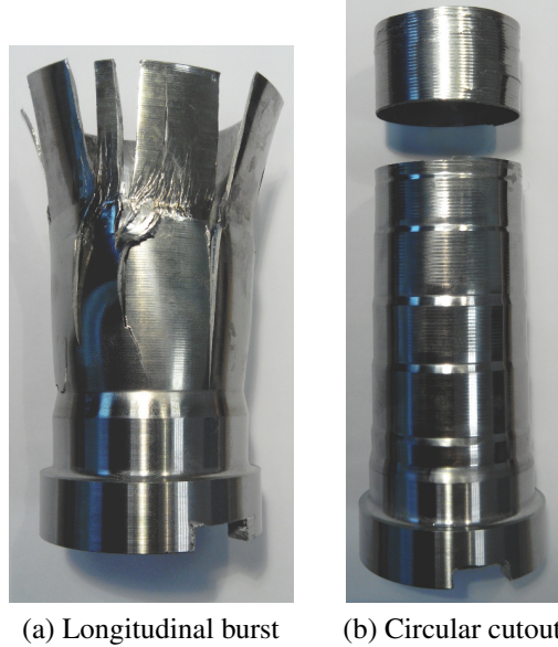
Fig. 3: Typical fracture patterns resulting from flowforming. Photograph (a) shows specimen 1, and Photograph (b) shows specimen 3.
