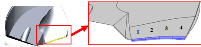
Fig. 6. Chip contact zone divided into four discrete regions for the mechanical and thermal simulations.
