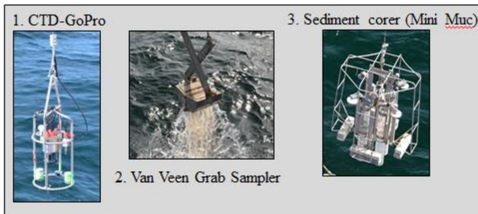
Figure 11: Altered sampling sequence for sediment observation via a CTD equipped with an underwater camera (GoPro).
