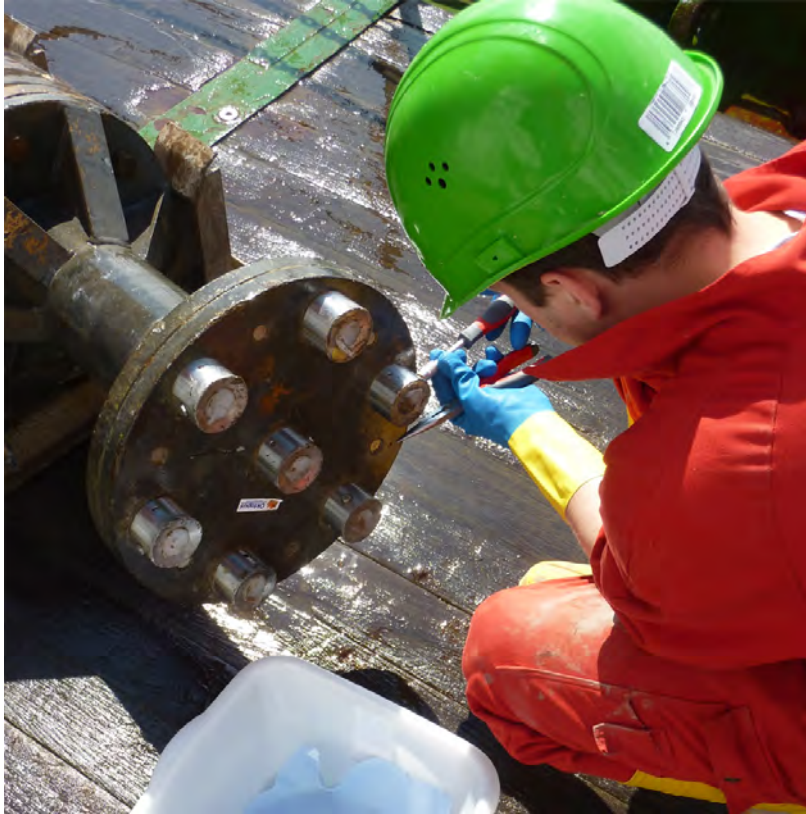
Fig. 14: Master Student Phillip Kosbü (University of Kiel) replacing the wax filled cups mounted around the crusher plate of the wax corer during Exp. POS511 (Photo: J. Geldmacher).
