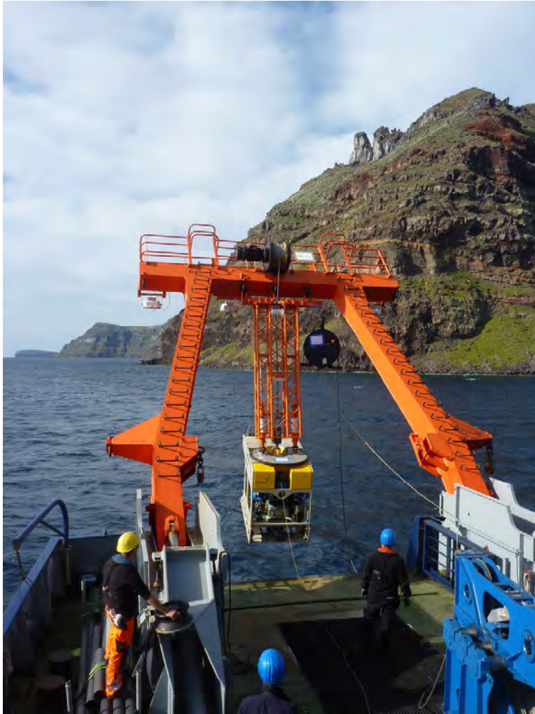
Fig. 6: ROV PHOCA being launched from RV Poseidon in the caldera of Santorini (off Cape Simandiri, Therasia Island). Foto: J. Geldmacher, GEOMAR
