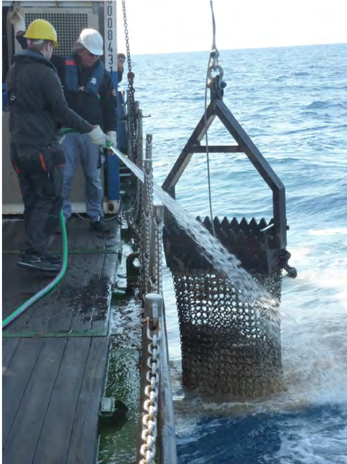
Fig. 13: A returning chain sack dredge (DR-13) full of heavy mud hanging off the portside deck of the POSEIDON (Photo: J. Geldmacher).
