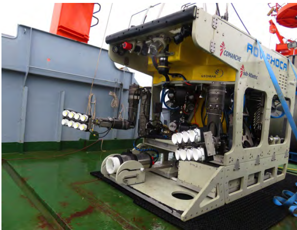
Fig. 7: Photogrammetry setup with DeepSurveyCam on starboard drawer and two flashlight arrays in the manipulator arms. Photo: ROV-Team, GEOMAR
