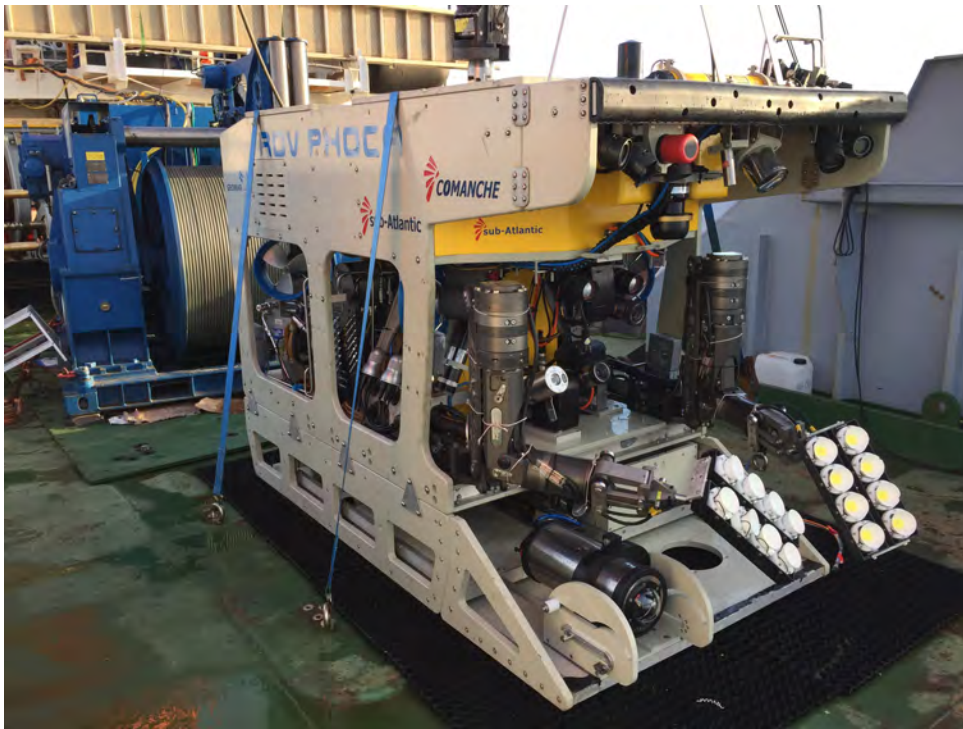
Fig. 10: ROV Phoca with the DeepSurveyCam mounted on the front porch (Photo: Kwasnitschka, GEOMAR).
