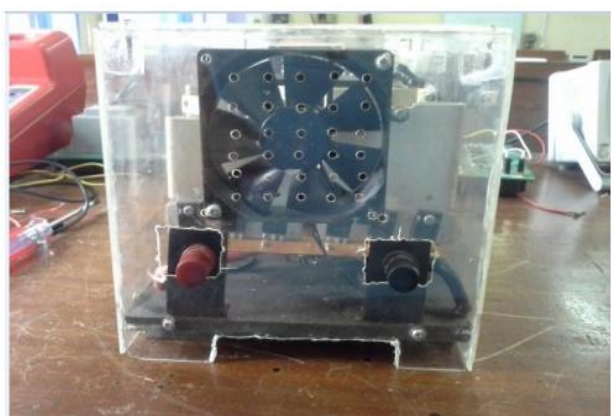
Figure 9: Side View of the Inverter System showing DC Fan and Battery Terminals
