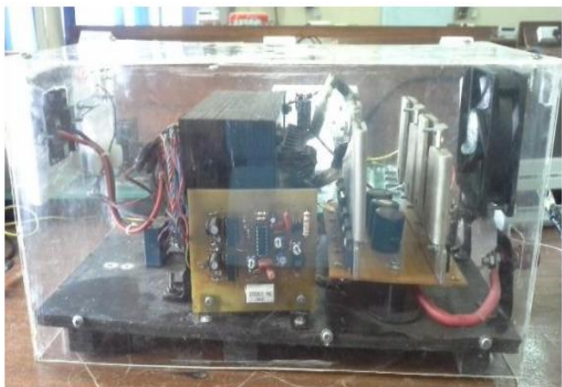
Figure 8: Side View of the Inverter System showing the Oscillator Circuit, the Transformer and the H-Bridge
