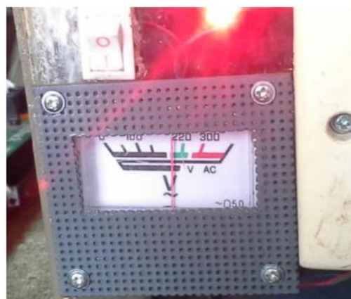
Figure 13: Output Voltage Reading of the No-Load Test
