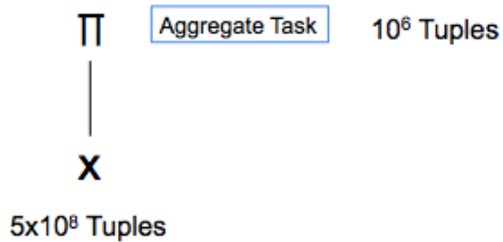
Figure 5.4: Output Size Estimation of Vector/Matrix-Based Implementation of Gram Matrix Computation. (The Column number of X is 1000)
