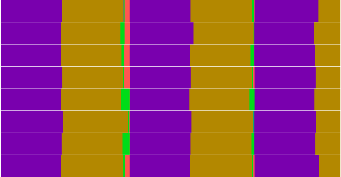
Figure 3.12: Trace graph of 1 second of running time, 8 cores, generated by the HPCTOOLKIT [ABF + 10]. The horizontal axis is the time axis. Eight horizontal rows represent computation timing of eight cores. The top row is for the first time subdomain, etc. One optimization iteration consists of two major blocks, one purple and one brown. The purple blocks are for forward computation, the brown blocks are for backward computation. The smaller green and red blocks correspond to communication and error estimation timing respectively.
