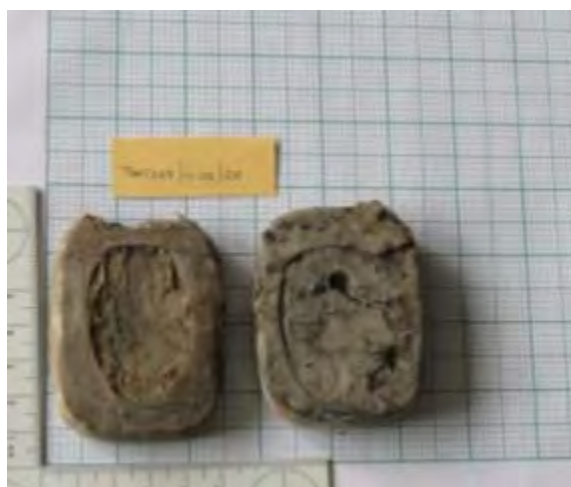
Figure 5.121: Fragments from an Eveready 9v transistor battery. (Photo: Author's own).
