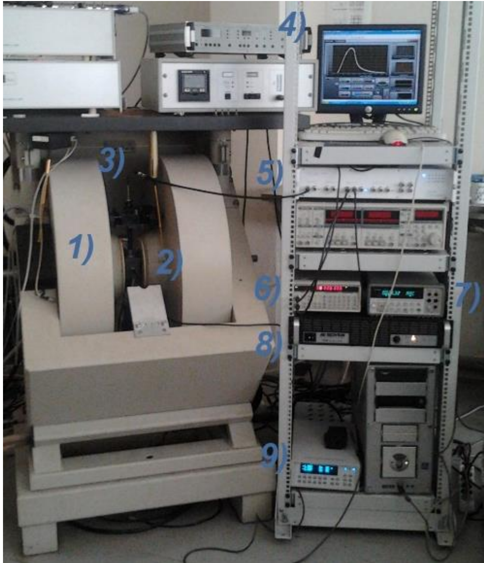
Figure 3.2 Photo of the setup used in the ME measurements. The labeled components are: 1) electromagnet (from the Bruker® ESP 300E spectrometer); 2) box containing the Helmholtz coil; 3) sample support and goniometer; 4) PC; 5) lock-in amplifier (Zurich Instruments®, model HF2LI); 6) function generator (SRS®, model DS345); 7) multimeter (Agilent®, model 34401A); 8) power amplifier (AE Techron®, model 7224) and 9) gaussmeter (DSP®, model 475).
