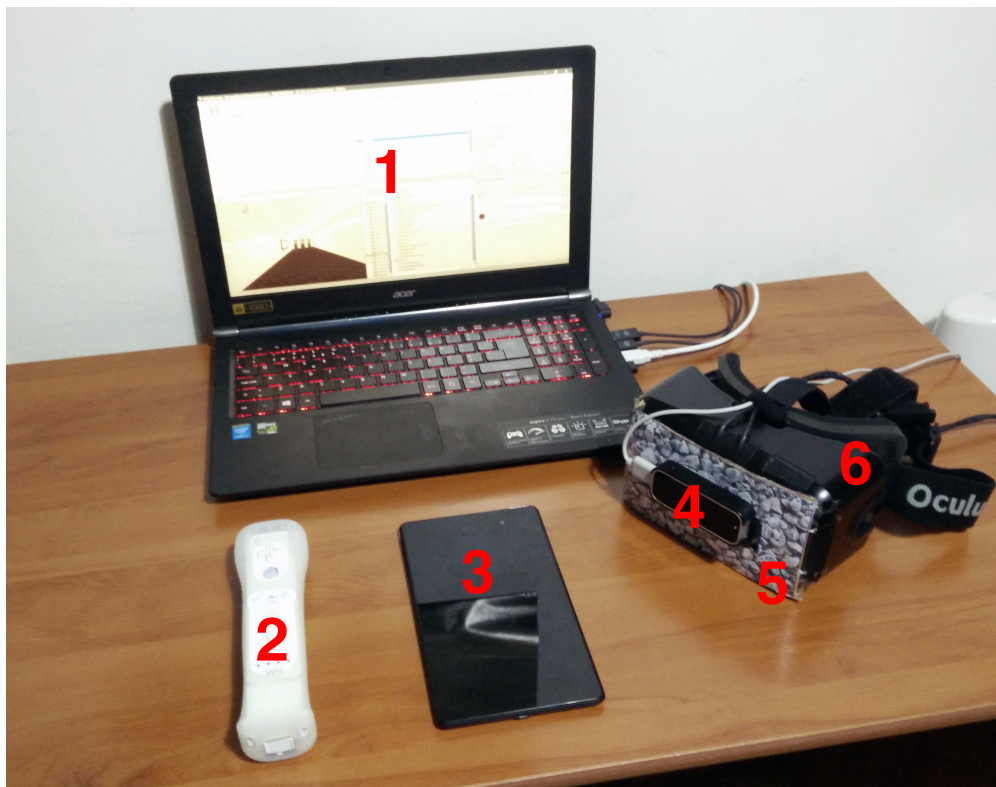
Figure 4.3: Hardware setup. 1) Computer running the main application; 2) Wiimote controller; 3) Tablet (Nexus 7) running the tablet application; 4) Leap Motion Controller connected to the computer; 5) Augmented Reality marker attached to the Oculus Rift DK2, Oculus Rift DK2: virtual reality headset, connected to the computer
