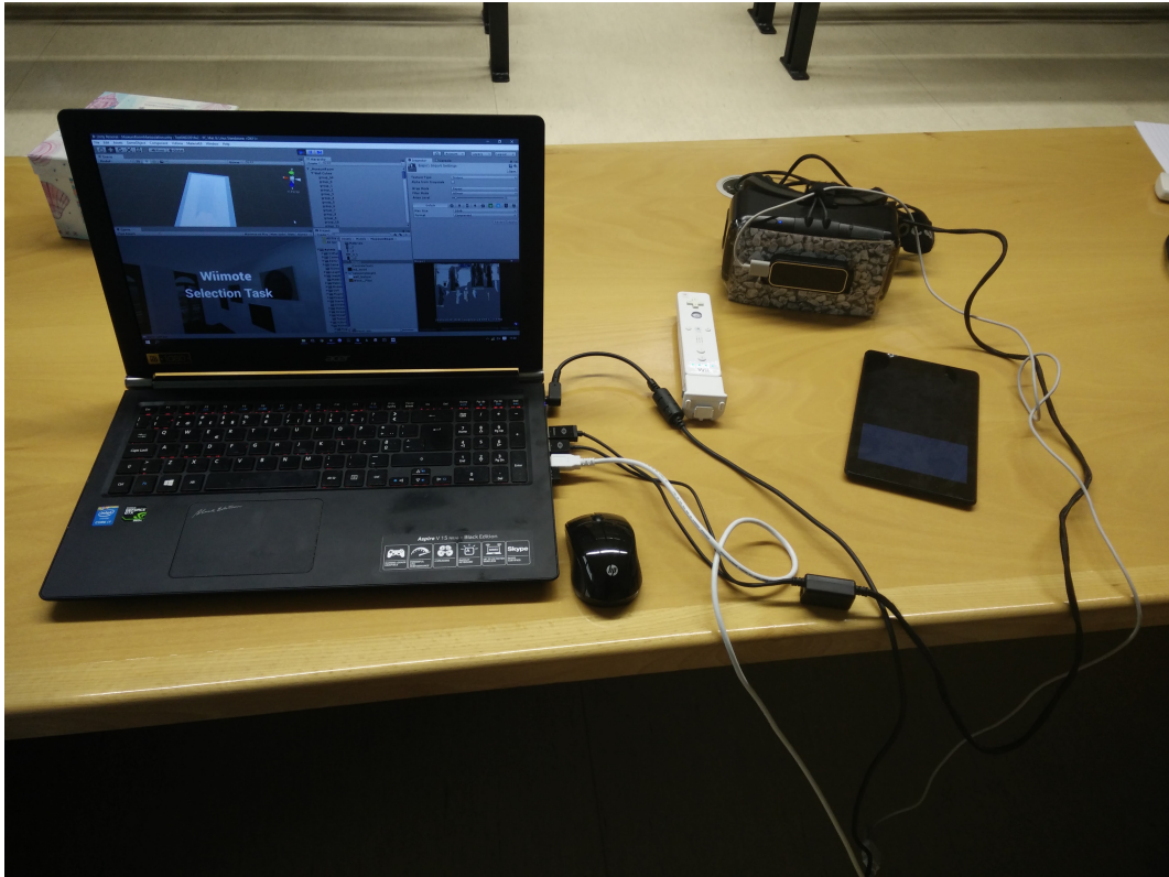
Figure 6.9: Experiment setup: Laptop computer; Wiimote; Nexus 7 Tablet; Oculus Rift DK2; Leap Motion Sensor (mounted on the Oculus Rift)
