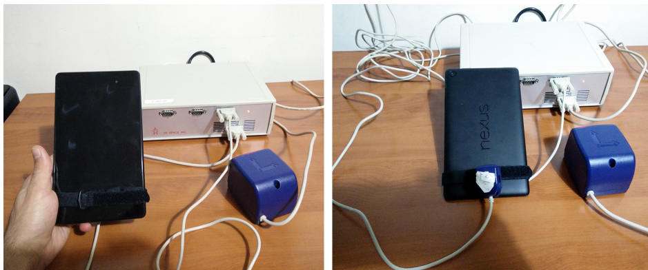
Figure 4.4: WinTracker III - Virtual Reality Tracker attached to the Nexus 7 tablet
