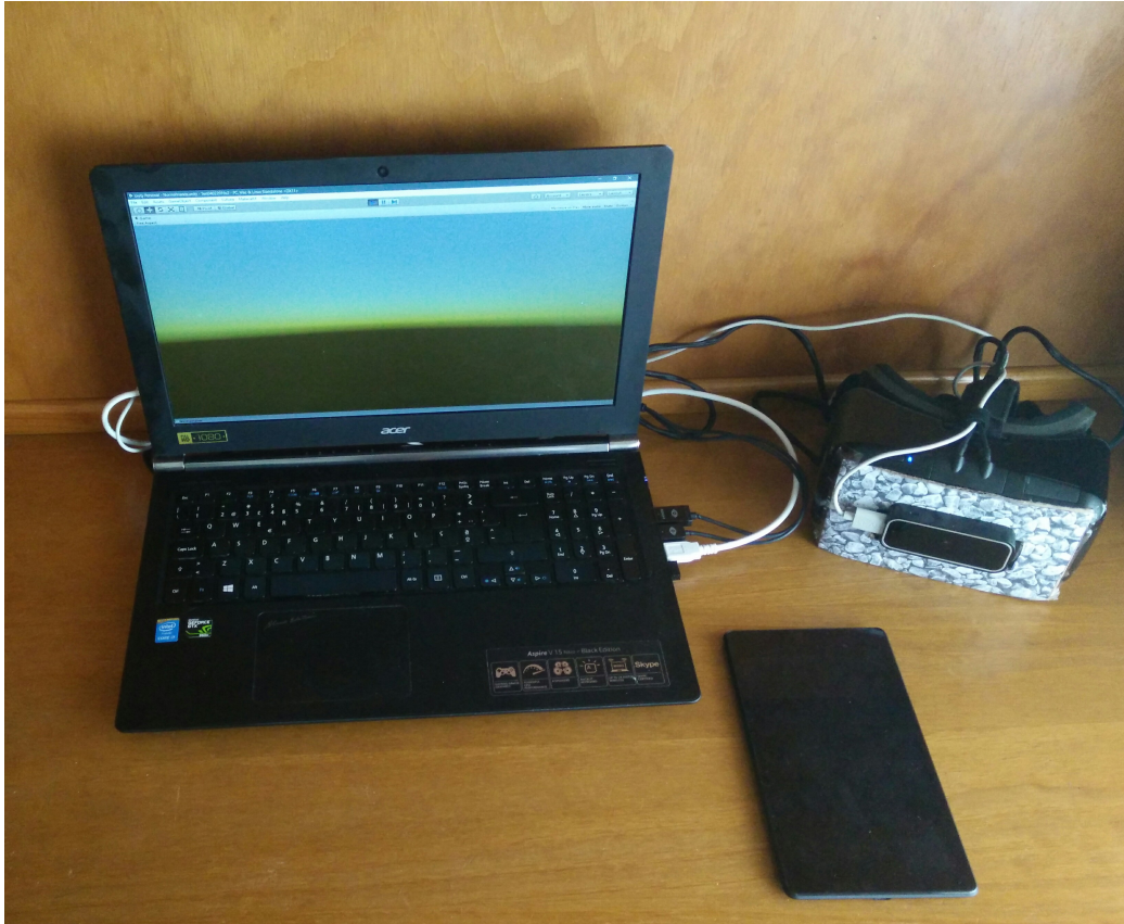
Figure 6.4: Experimental setup: Laptop computer running the Unity application; Nexus 7 Tablet; Oculus Rift DK2; Leap Motion Sensor (mounted on the Oculus Rift)
