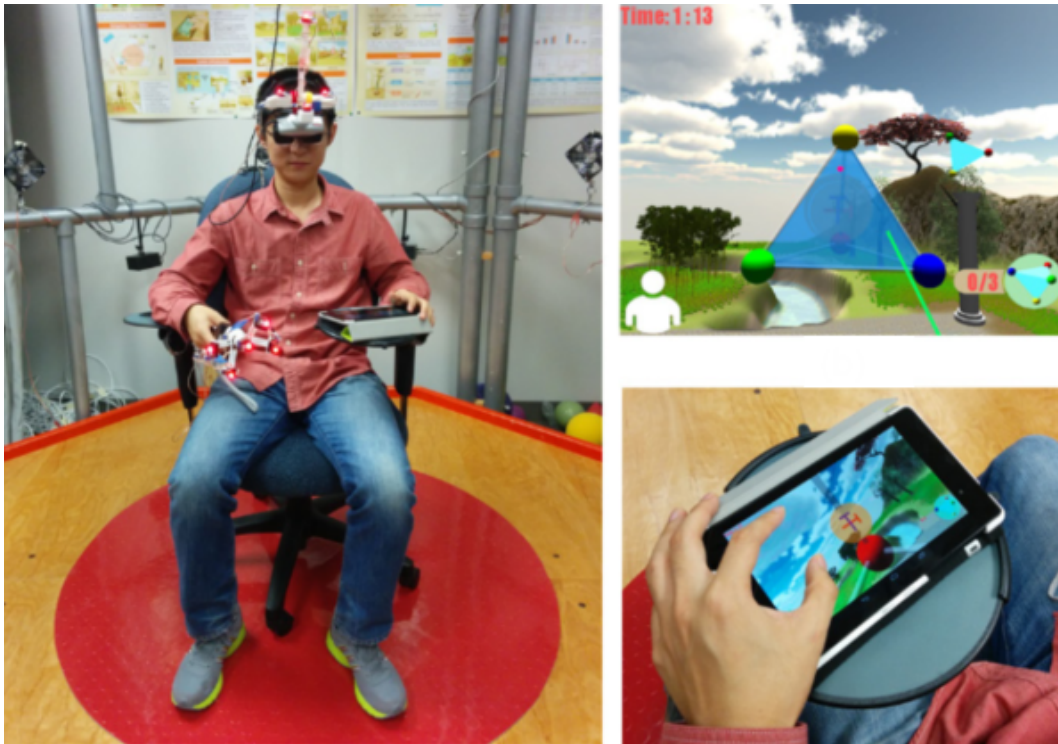
Figure 2.17: On the left: The hardware setup of the HVE system; On the top right: user’s virtual avatar view on the HMD; On the bottom right: the objects view on the tablet. ([Wang and Lindeman, 2015])
