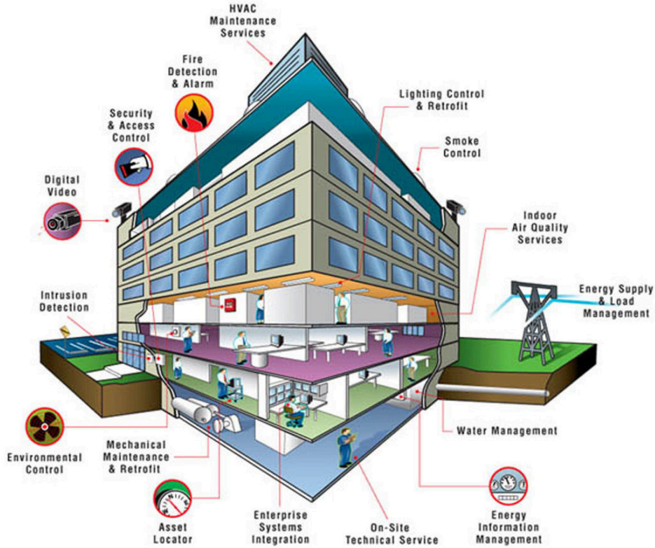
Figure 2.1: Building services in a Building Automation System [8].
