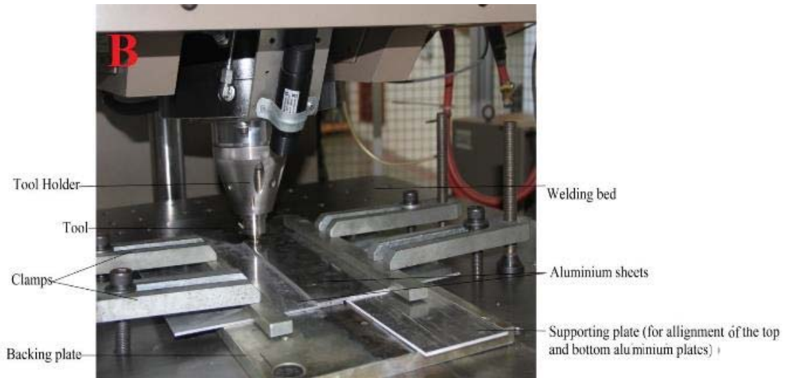
Figure 3 Experimental weld setup of FSW platform
