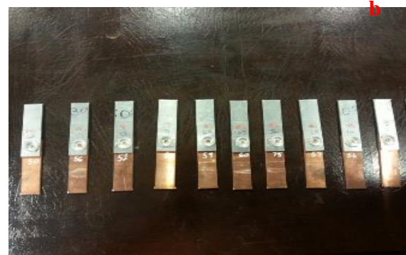
Figure 1. Depicts the I-STIR friction-stir welding machine (a) and geometry of the lap shear tensile sample (b).
