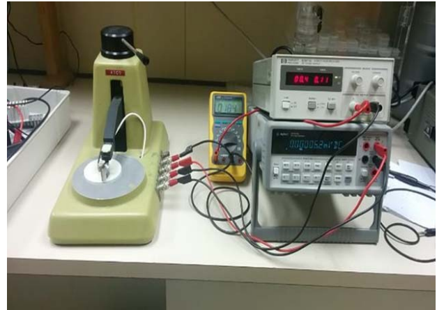
Figure 2. Experimental set-up for electrical resistance measurement
