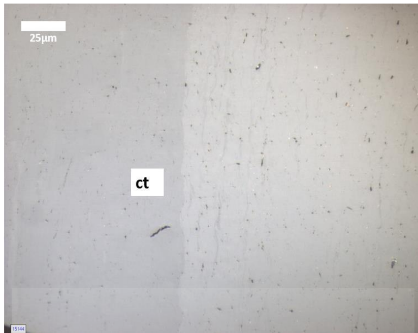
Figure 4.18: Photomicrographs of collotelinite on the left showing a slight higher reflectance compared to collotelinite on the right (15154). (Reflected white light, oil immersion, x500).
