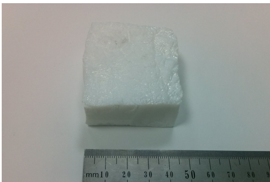
Figure 14. Alumina nanofibers in as received form. The diameter of the fibers was 10–40 nm.
