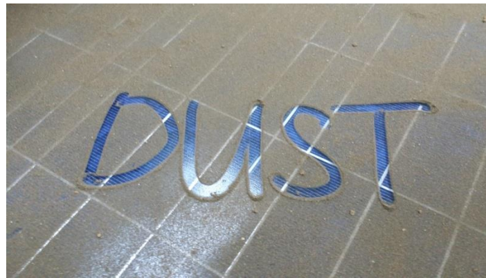
Figure 1: Accumulated Dust or Soiling on PV Module's Surface
