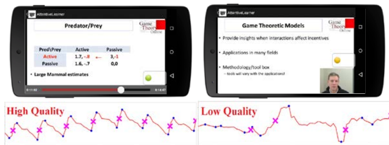
Figure 27. Top: Screenshots of AttentiveLearner in the experiment. Bottom: PPG signal at the time of the screenshot. Left: high-quality PPG, right: low-quality PPG.
