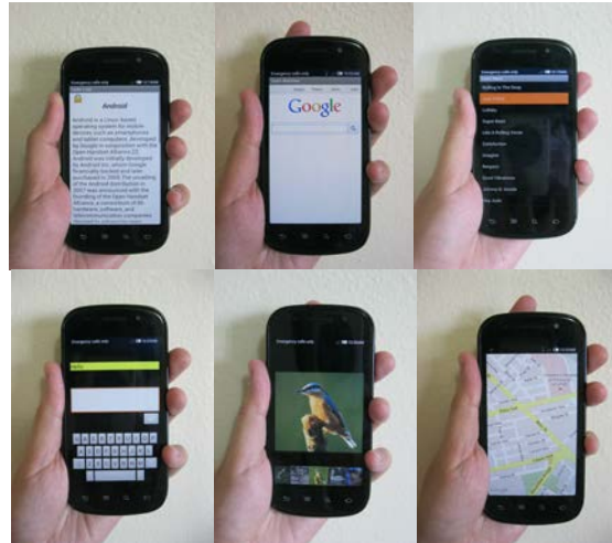
Figure 12. Sample LensGesture applications. From left to right, top to bottom - LensLock, LensCapture, LensMenu, LensQWERTY, LensAlbum, and LensMap.
