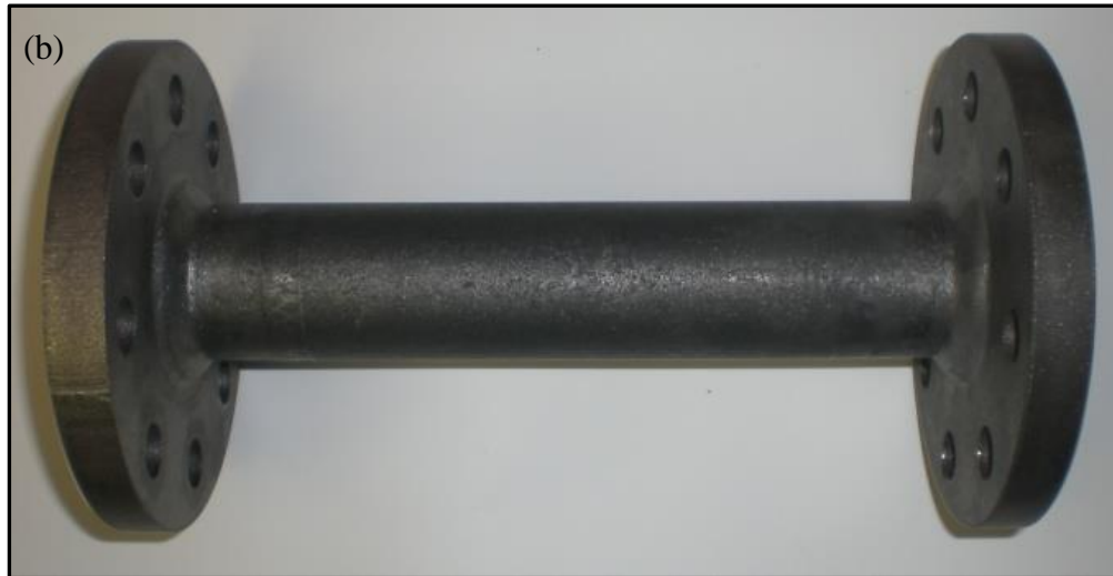
Figure 6.5.5: (a) Geometry and nominal dimensions of tube-to-flange structural steel welded joints used in the experimental tests under torsion loading. The specimens were arc-welded with fillet-welds. (b) An example of tube-to-flange specimen.
