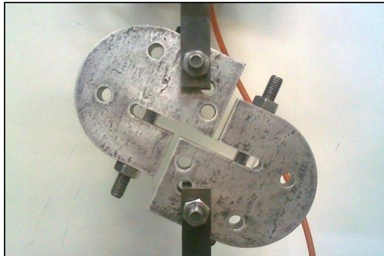
Figure 2.3.4. The test configuration used for fracture tests on PMMA.
