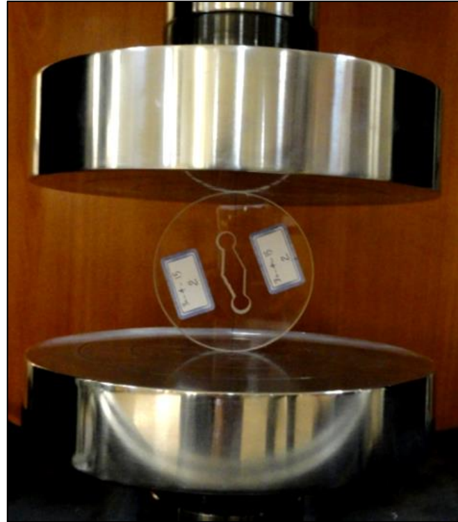
Figure 2.1.6. A VO-BD specimen subjected to mixed mode I+II loading inside the test machine.
