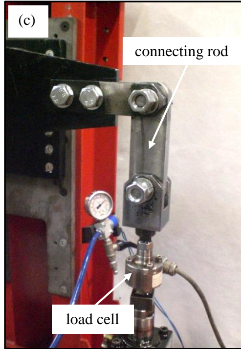
Figure 6.5.6: (a) Test rig for pure torsion fatigue loading. (b) Pneumatic system used to monitor the number of cycles to break through. (c) A detail of the connecting rod between the servo-hydraulic actuator and the lever arm.
