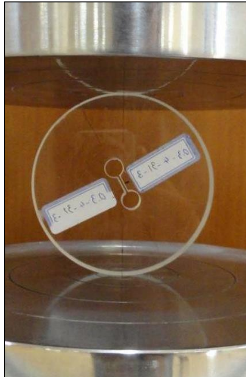
Figure 2.1.3. A Key-BD specimen under mixed mode I+II fracture test.
