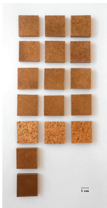
Figure 2. Test specimens of the binderless fiberboards produced during this study. Row 1–4, Fiberboards produced from extrusion refined straw with a L/S ratio of 1.0, 0.8, 0.6 and 0.4, respectively; Row 5, Fiberboards produced from milled straw; Columns 1–3, Fiberboards produced with a press cake content of 10%, 25% and 40%, respectively; Row 6, Fiberboard produced from premixed extrusion refined straw at L/S ratio 0.4 and 40% of press cake; Row 7, Fiberboard produced from premixed extrusion refined straw at L/S ratio 0.4 and 40% of press cake and subsequently heat treated at 200 °C.
