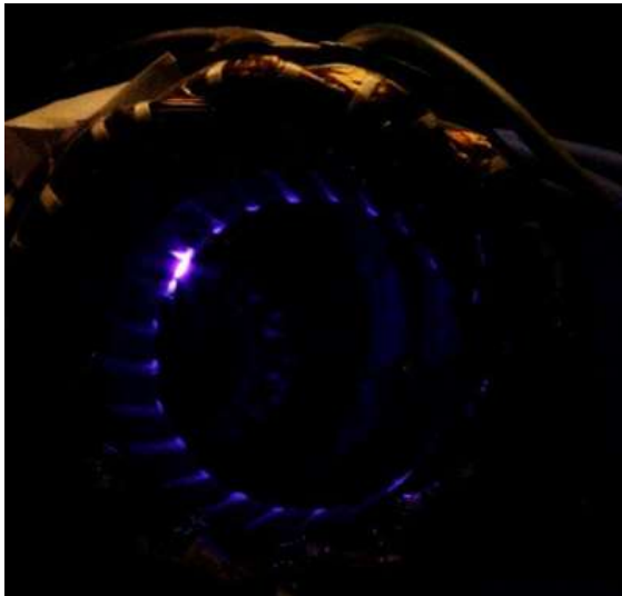
Figure I.8: Partial discharges in the slot (100 mbar)
