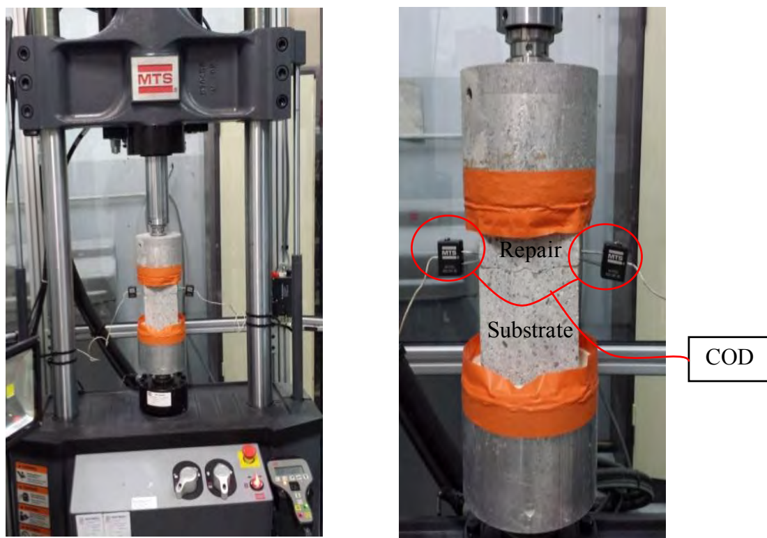
Figure IV-18: Complete experimental testing set-up for determining interfacial bond strength degradation
