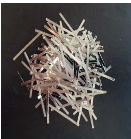
Figure II-1: Amorphous metallic fibers of 30mm length
