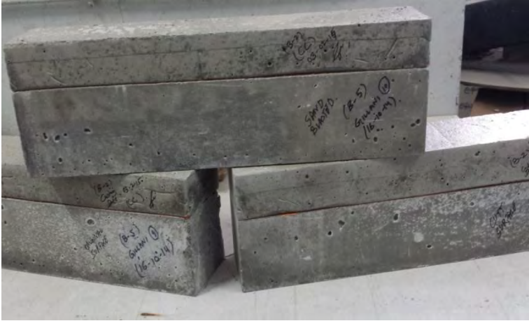
Figure III-8: Specimen after repair casting
