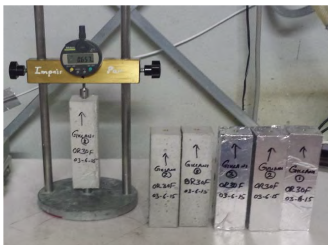
Figure II-16: Apparatus for shrinkage measurement
