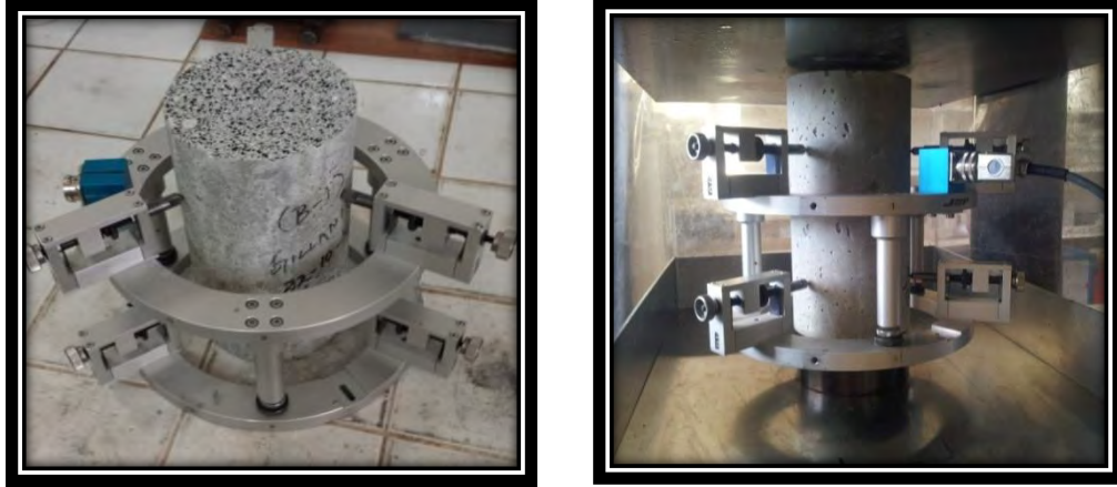
Figure II-5: Testing set-up for compressive modulus of elasticity
