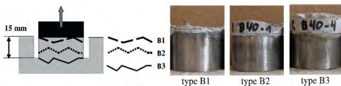
Figure I-18: Failure modes on pull-off test scheme for surface tensile strength evaluation and examples of type B1 [superficial], B2 [middle] and B3 [deep] self defined failure modes (L. Courard et al., 2014)
