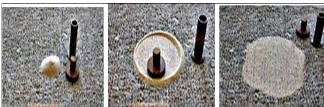
Figure I-17: Sand test for surface roughness evaluation (L. Courard et al., 2014)
