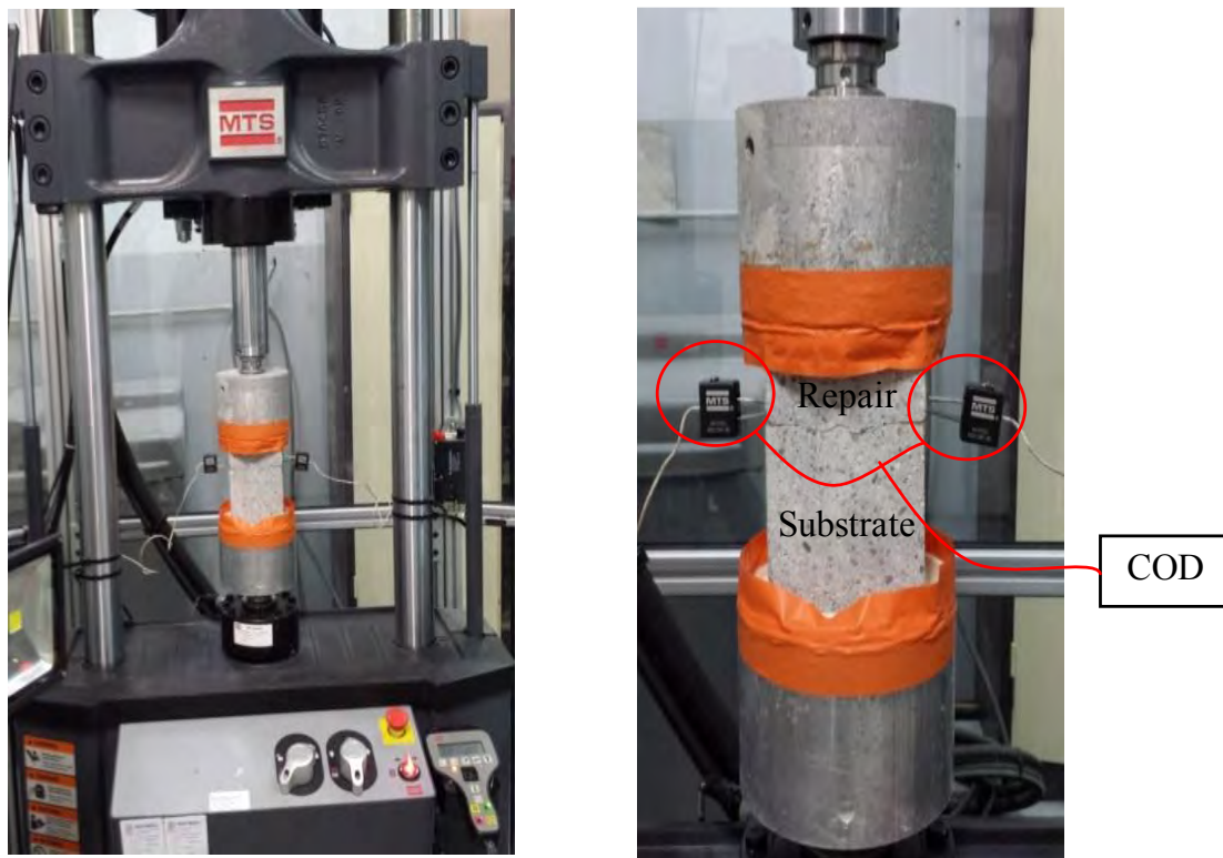
Figure III-10: View of notched specimen for bond tensile tests controlled by COD
