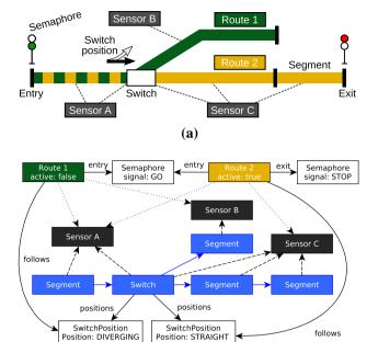
Fig. 1 Domain concepts of the Train Benchmark. a Illustration for the concepts in the Train Benchmark models. b The concepts as a typed property graph
