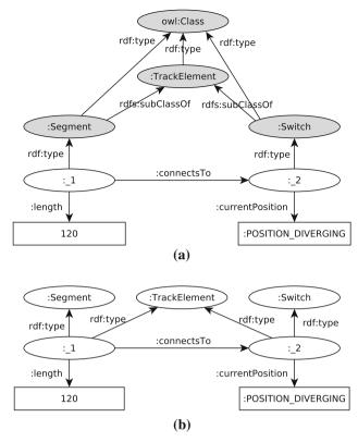
**Fig. 5** RDF instance models. **a** An RDF instance model *with metamodel*. The vertices for the (relevant part of the) metamodel are depicted in *gray*. **b** An RDF instance model *with inferred triples*. Note that the inferred edges to TrackElement node are explicitly asserted in the model
