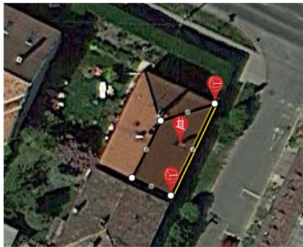
Fig. 5. Initial boundary conditions of the auto-sizing based on Google Maps API
