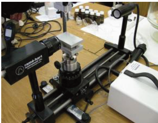
Figure 3. SEE System apparatus which used to evaluate the contact angle of polymer
