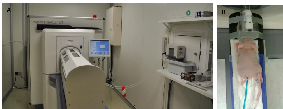
Figure 15: SPECT-CT preclinical imaging system from GE installed in CIC biomaGUNE (A) and animal positioned on the SPECT-CT gantry (B).
