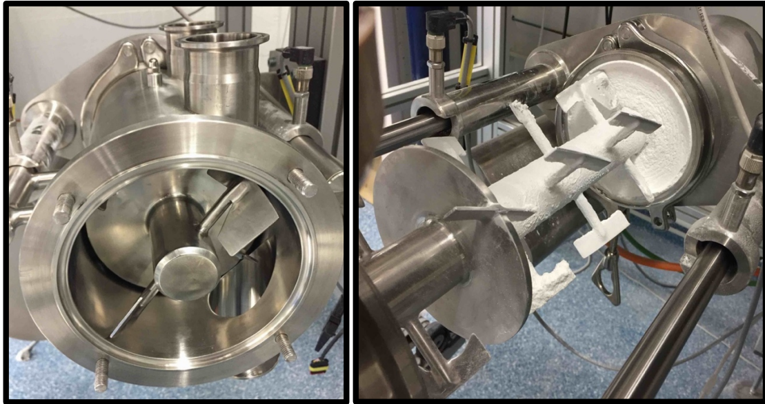
Figure 16 - Modulomix in-line mixer. On the left: With the side panel removed, exposing the mixing chamber. On the right: Before cleaning with the external casing removed
