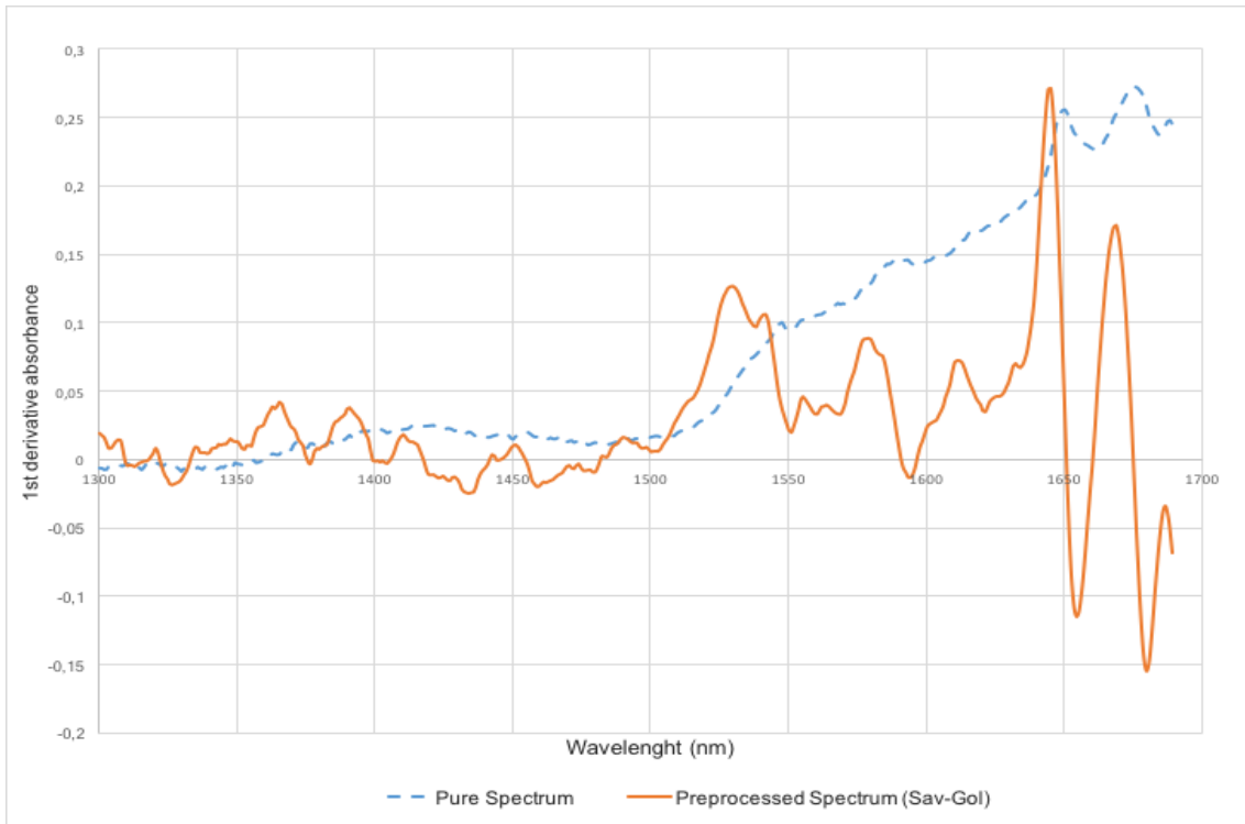
Figure 28 - Raw and preprocessed (first derivative) NIR spectra of paracetamol.
