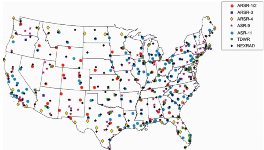
FIG. 1. Locations of U.S. operational weather and air traffic control radars.
