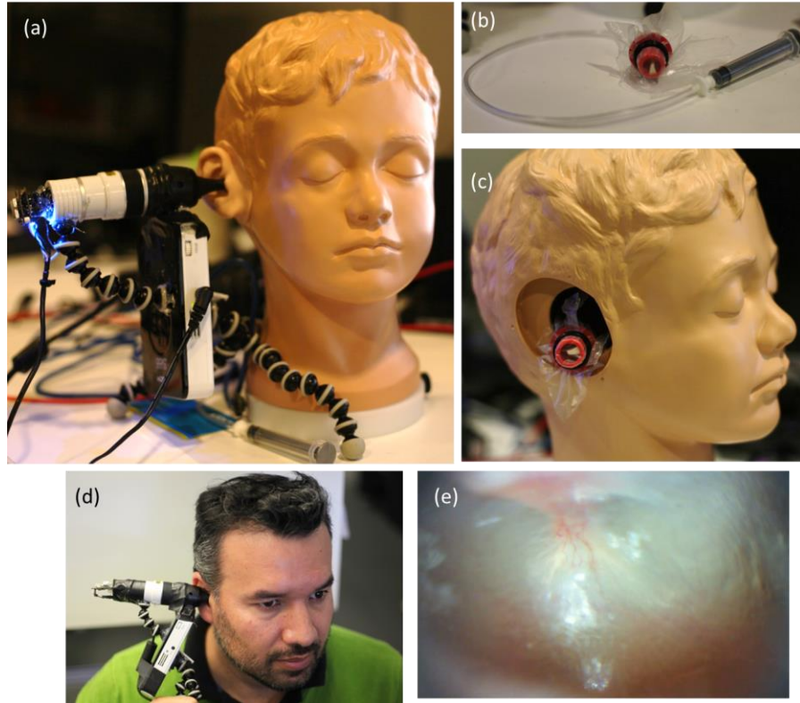
Fig. 2 (a) The prototype being tested on the ear phantom arrangement. (b) A syringe attached to the ear drum cartridge that was used to vary pressure. (c) The TM phantom placed in the ear cavity. (d) Photograph of the prototype being tested on a volunteer. (e) A typical picture of the TM captured by the device under regular illumination.
