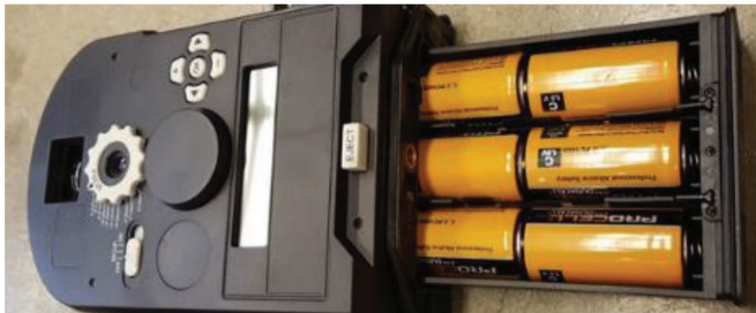
(e) Time-lapse camera takes C-cell batteries
