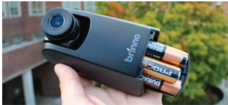
(e) Time-lapse camera takes AA-cell batteries, accessible from bottom
