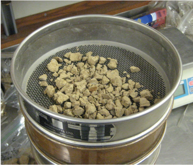
Figure 5.2 Photograph of the soil before starting the wet sieving process.
