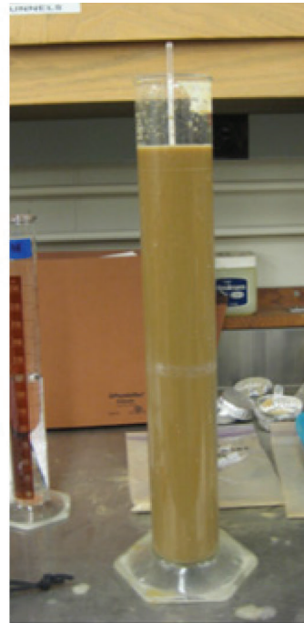
Figure 5.4 A photograph, on the left, of the soil solution being amalgamated with the electric mixer and a photograph, on the right, of the hydrometer placed in the soil solution.
