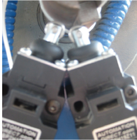
Figure 3.6 Ending position limit switch engaged.
