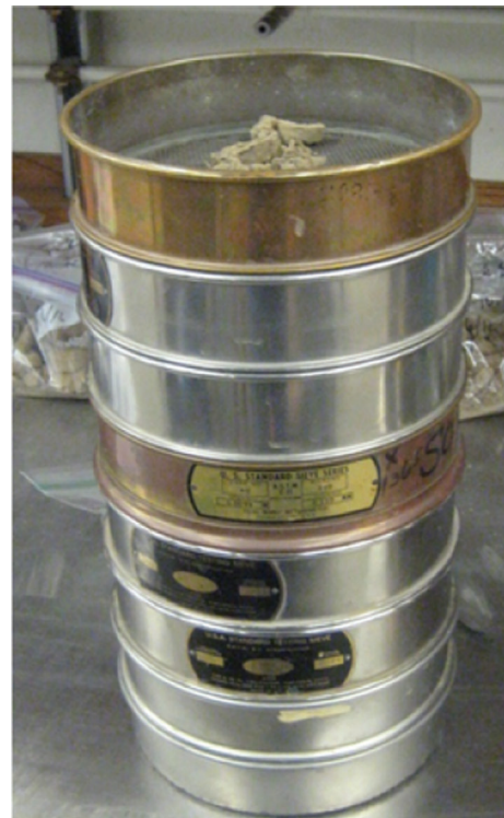
Figure 5.1 Photograph of a sieve set used to determine the soil gradation.
