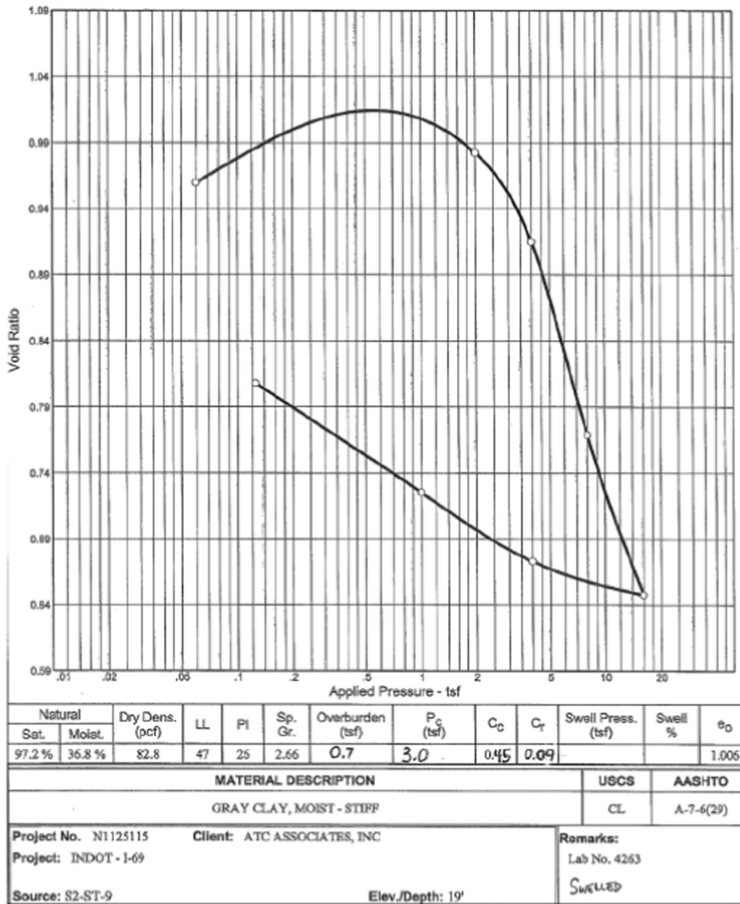
Figure C.23 1-D consolidation test from the Kolen site performed by INDOT.
